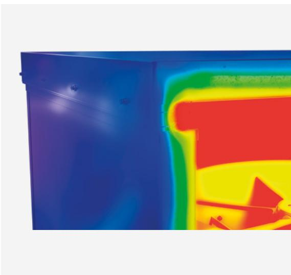
The new **HATCH/HP** has an extraordinarily low thermal transmittance coefficient:
